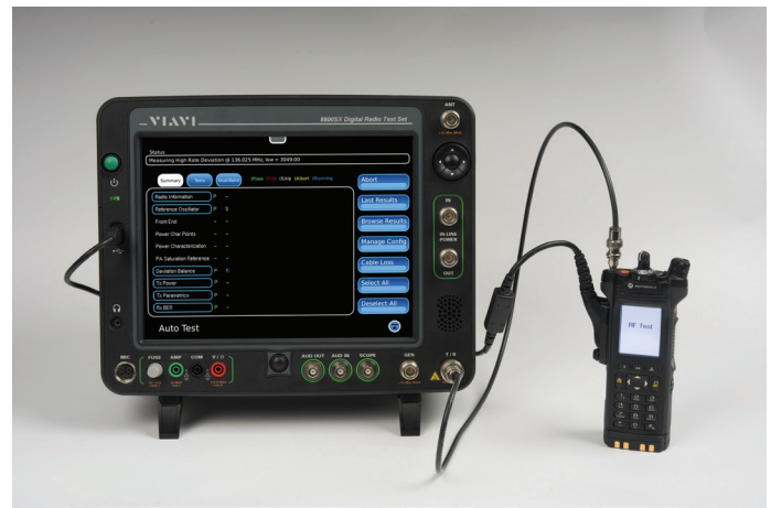
The 8800SX Auto-Test Setup
